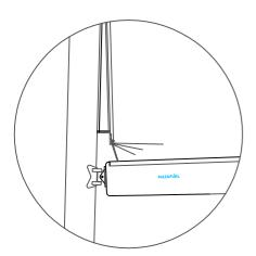
The main should work back gradually as it is furled. If the sail show stretch wringles, reduce the resistance on the halyard.
